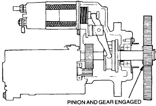
**Figure 76 Ignition Switch in START**
