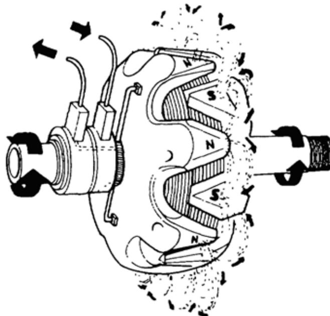
**Figure 79 Rotor and Magnetic Field**
