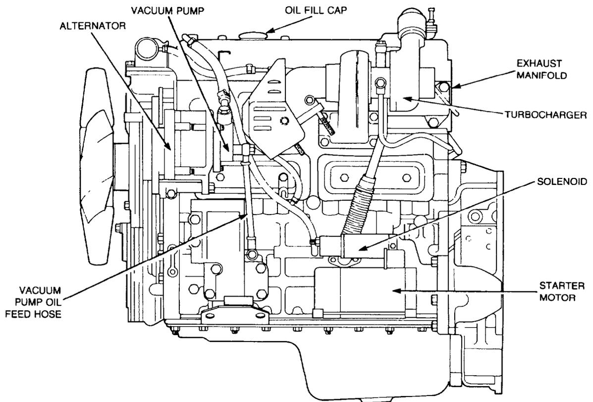
Figure 4 Isuzu Engine 4BD1T, Left-hand Side
