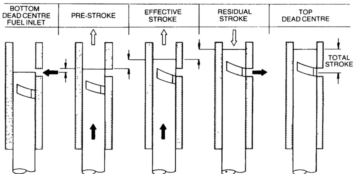
**Figure 22 Phases (Strokes) of the Plunger**
